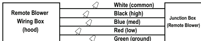
CBE-1000 / PBN-1000A: WIRING DIAGRAM
