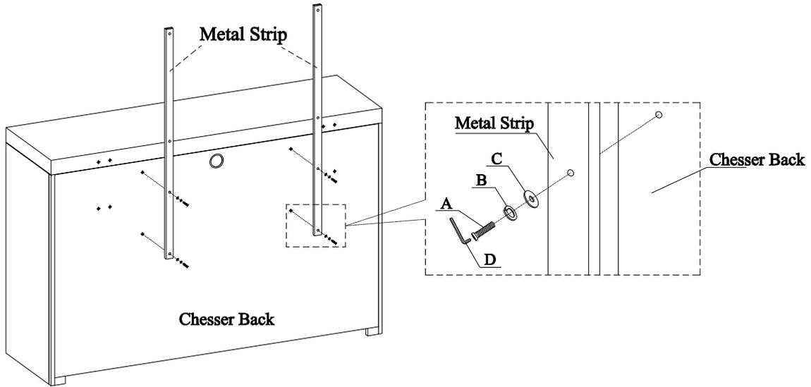
**STEP 2:** Attach the metal strips to the TV frame by using 4 bolts (A), lock washers (B) and flat washers (C). Tighten all the bolts on TV frame and Chesser with Allen wrench.
