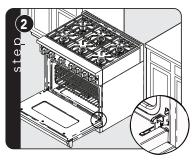
Fold latches backward until locked in place.
