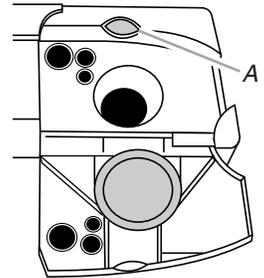
**NOTE:** For most water conditions, the factory setting of 2 will give good results. If you have hard water or notice rings or spots, try a higher setting. Turn the arrow adjuster inside the dispenser by either using your fingers or inserting a flat-blade screwdriver into the center of the arrow and turning.
