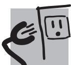
**Do not, under any circumstances, cut or remove the third (ground) prong from the power cord. For personal safety, this appliance must be properly grounded.**
