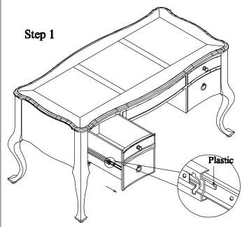
Press the left side plastic up, and press the right side plastic down, then pull out the drawer.
