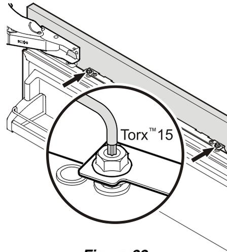
2. Open the refrigerator door and hang the panel on the top adjusting bolts (**Figure 31**).
