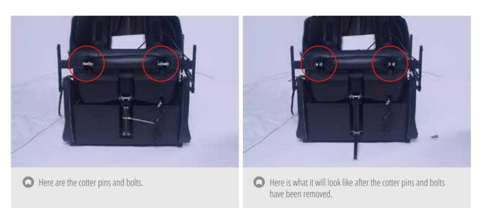
**Connect footrest to base.** Move the footrest close to the chair. Engage the link rod with the footrest joint, then insert the bolt and lock with the cotter pin.
