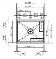
C.O. 18" (457 mm) 1/2" (13 mm ) REVEAL FRONT AND BACK 10"(254 r I.D. 16" (406 mm)
