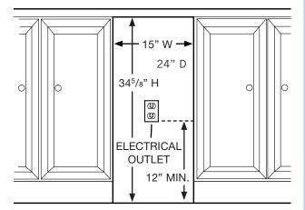
The compactor requires an under-counter opening 15-in. wide, 34<sup>5</sup>/<sub>8</sub>-in. high, and 24-in. deep.
