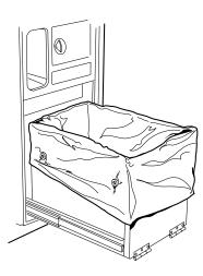
Smooth and shape the bag carefully this will prevent the bag from being torn by the ram during compaction.
