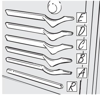
The oven has 5 rack positions. It also has a special lower rack position (R) for extra large items, such as a large turkey.
