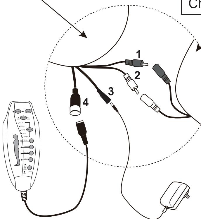
Wire 1: RED wire from the backrest connect to the RED wire from the seat.
