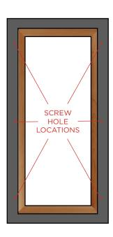
If readjustment is necessary loosen all 6 screws, reposition the panel and re-tighten the screws.
