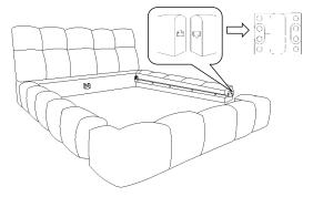
4. Metal connectors are preinstalled at the end of the side rails and footboard. Connect by sliding the two connectors together by overlaying them on top of each other.
