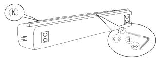
2. Feet for side rails are preinstalled. Use washers (G-2) with bolts (H) and attach slat support (K) with wrench provided (G-3). Screw and secure bolts tightly.
