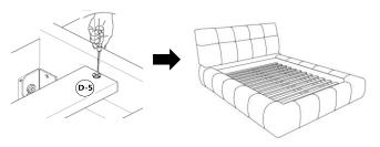
6.Open the rolled slats (D) and place on top of the slat support. Secure the slats using the screws (I).
