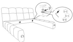
3. Secure connection of the headboard and side rails with brackets (F)and hardware provided(G1, G2, G3). Place and align bracket to the predrill holes. Insert bolts with washers and screw bolts tightly.
