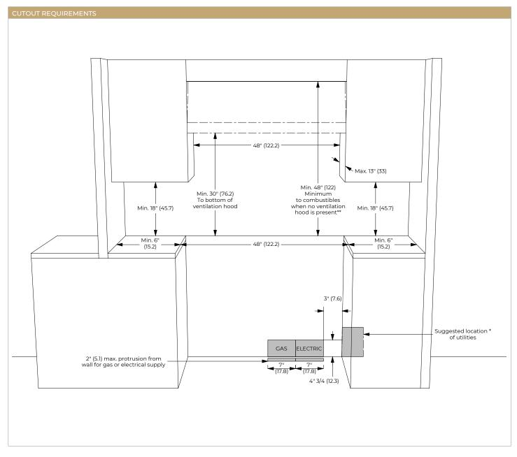
\*\*NOTE: Ensure your installation also complies with local and national building and fire codes. If the surface of the entire back wall above the range and below the hood is not composed of a non-combustible material then the 9" accessory back guard must be used. \*Consult local code for exact location requirements.
