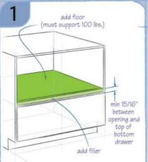
Remove top two drawers and slides. Add filler and support surface. Must support 100 lbs.
