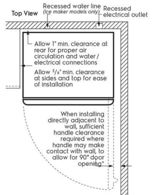
\* When installing refrigerator adjacent to wall, cabinet or other appliance that extends beyond front edge of unit, 20" minimum clearance recommended to allow for optimum 140° door swing, providing complete crisper access and removal. (Absolute 3" minimum clearance will ONLY allow for 90° door swing which will provide limited crisper access with restricted removal.)
