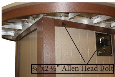
Fasten Firepit Top to Firepit Base by inserting 1/4" x 2 1/2" Allen Head Bolts into pre-drilled holes in frame and base (please note to keep bolt head on outside of base and fasten frame opposite side of door first) and fasten with 1/4" flange nuts.
