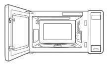
or a mild soap; rinse thoroughly with hot water. NEVER SPRAY OVEN CLEANERS DIRECTLY ONTO ANY PART OF THE MICROWAVE OVEN.
