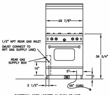
ELECTRICAL CORD LOCATED IN BACK OF UNIT LOCATION OF ELECTRICAL OUTLET MUST NOT BE HIGHER THAN 3" FROM FLOOR IF LOCATED BEHIND THE UNIT OR CAN BE LOCATED IN AN ADJOINING CABINET.
