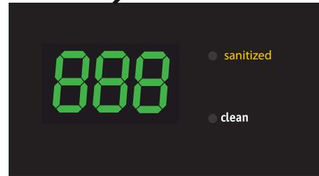
PF..... Appears in window when dishwasher is first installed, or when power has been interrupted. HI-TEMP WASH and NO HEAT DRY indicator lights will also flash. To clear, touch START/CANCEL pad.
