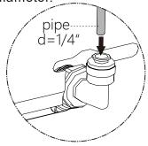
3. Put the blue clip back to the connector to lock the connection.
