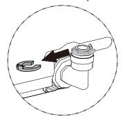
2. Take out the soft pipe from the freezer drawer, insert it into the connector and push it to the end, the soft pipe should be ¼ inch (6.35mm) in external diameter.
