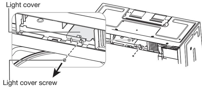
5. Open the light cover by removing the light cover screw, then carefully pull up on the front edge.
