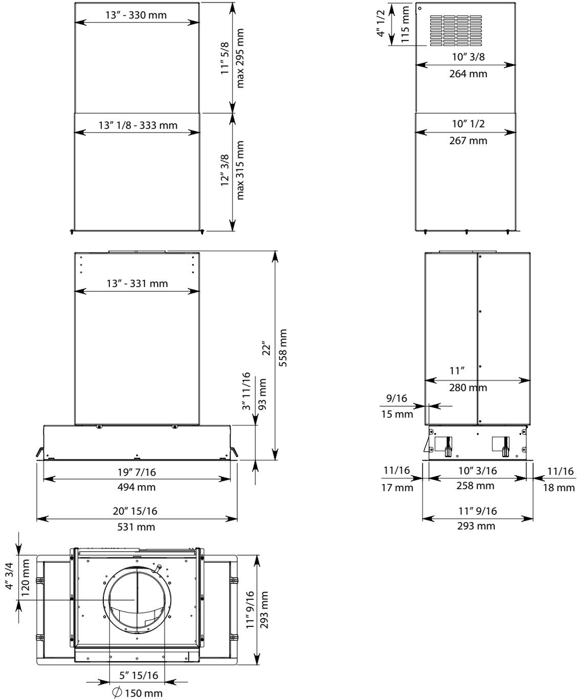
EN - Hole measurements for installation
