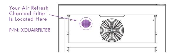
Rotate the filter 1/4 turn to unlock
