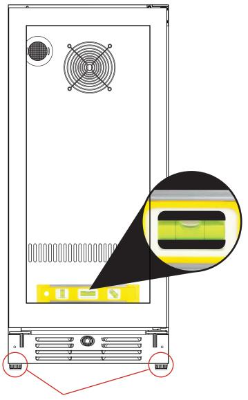
Rotate to raise or lower the LEVELING LEGS located at each of the four corners until all four legs are seated firmly on the floor and the interior floor of the unit is level both front to back and side to side.
