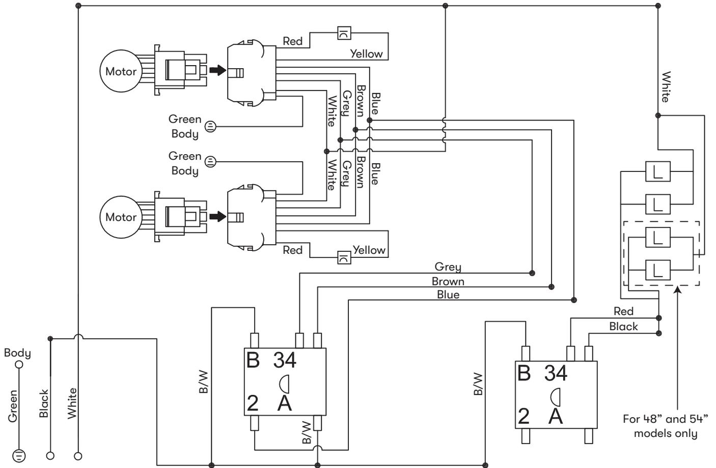
REMARKS: CONDENSER 22uF / 250VAC 2PCS FIT AC120V 60Hz
