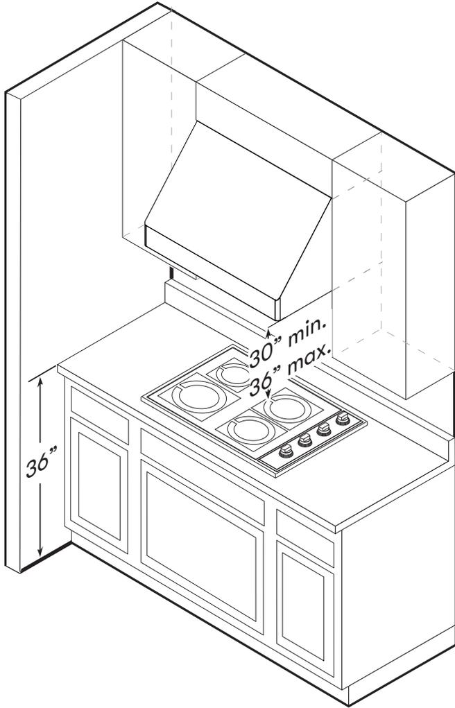
A minimum of 10" round duct is recommended to maintain maximum air flow efficiency.
