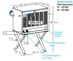
Voltage supply for ice maker and condensing unit are separate.
