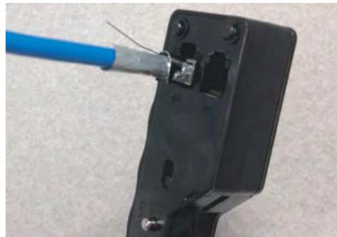
2. Crimp the external ground by placing the cable in the external ground crimping cavity and then pressing the handle.
