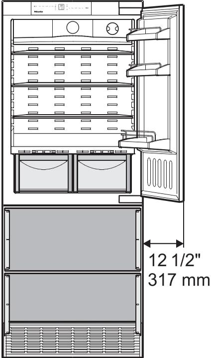
These measurements do not take the cabinet front and the door handle into account; they must be added on accordingly.
