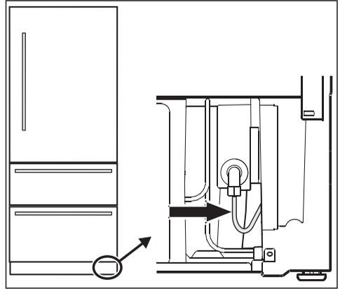
Water line feed-in (**D**) from left or right above the anti-tipping bracket.
