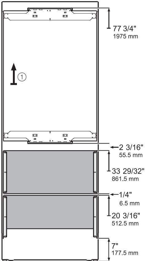
① This dimension line indicates the height measured from the floor.
