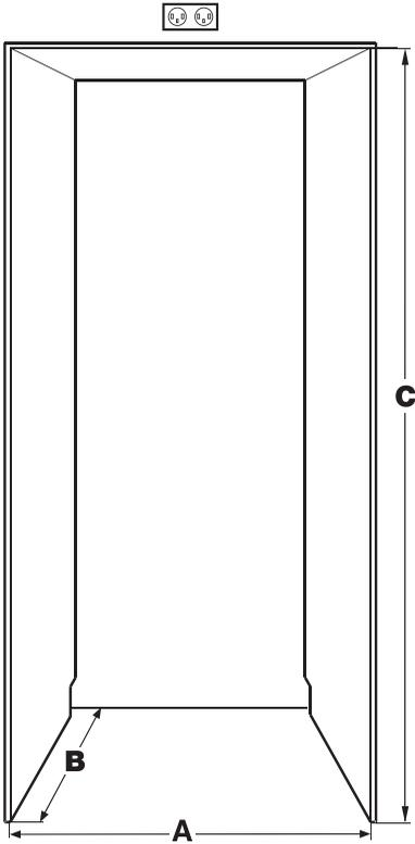
The location of the electrical outlet can be within a radius of 80" from the appliance top center. Do not install the electrical outlet **behind** the appliance!
