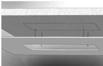
Make 4 holes in the ceiling according to the dimensions as shown in Fig. 4, place the metric plugs provided in the holes.
