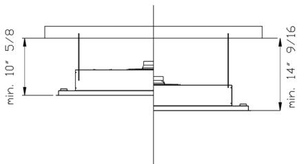
in case of a larger gap between the hood and the ceiling, you need to use longer threaded bars.
