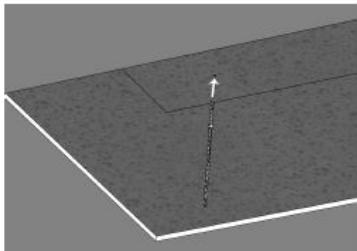
The threaded bars are 9"13/16 long and serve to install the ceiling-mounted hood at a distance from the solid ceiling of between 10"5/8 mm and 14"9/16 as shown in fig. 6.
