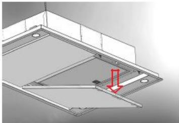
After having chosen the most suitable position, prepare the ducting: an air outlet connection piece, with a diameter of 6" to be installed in the side selected, is provided with the appliance.
