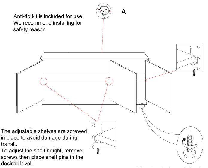
Adjust leveler if needed to level console on uneven floor.
