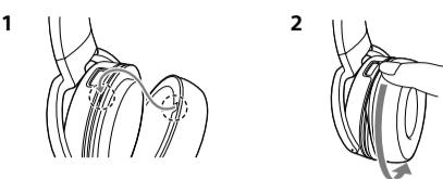
1 Align the projection in the groove on the main part with the notch on the earpad.
