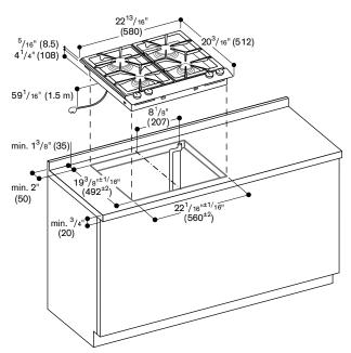
Minimum distance from the appliance cut-out to the side wall 11<sup>13</sup>/16" (300 mm).
