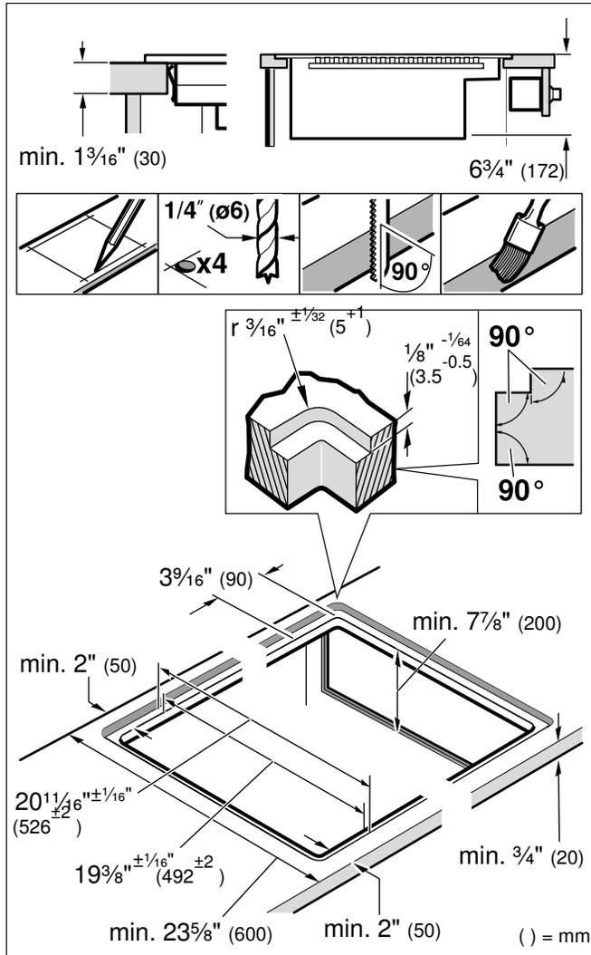
**Combining several Vario devices:** The connecting strip VA 420 000/001/010/011 is required for the combination of several Vario appliances. This is available separately as a special accessory. Consider additional space requirement for the connecting strip between the appliances when making the cut-out (see installation instructions VA 420 000/001/010/011).
