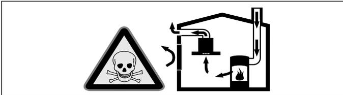
Room air-dependent heat-producing appliances (e.g. gas, oil, wood or coal-operated heaters, continuous flow heaters or water heaters) obtain combustion air from the room in which they are installed and discharge the exhaust gases into the open through an exhaust gas system (e.g. a chimney).
