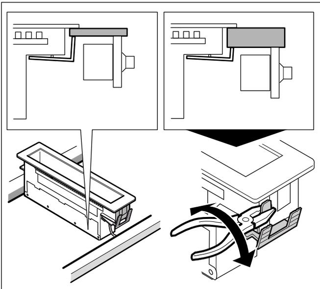
Insert and align the appliance in the cutout horizontally. Tighten the rear clamp using the screw inside the appliance. Tighten the front clamp from below.
