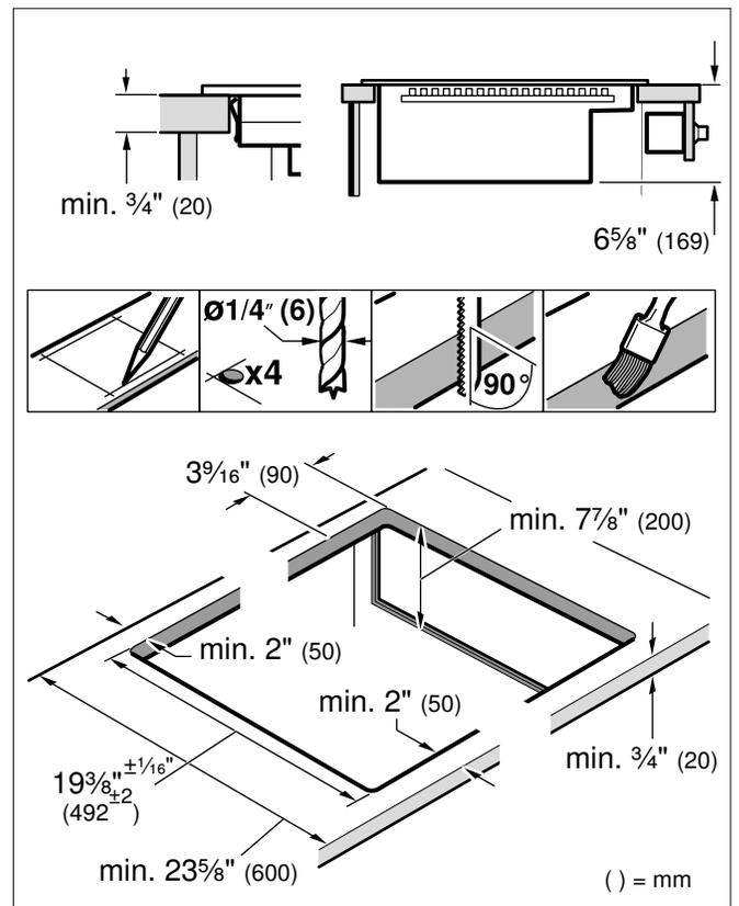
**Flush mounting:** Flush mounting into a countertop is possible.
