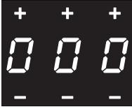
The first digit on the left is used to select the hours, the middle one to select the tens of minutes and the one on the right to select the minutes.
