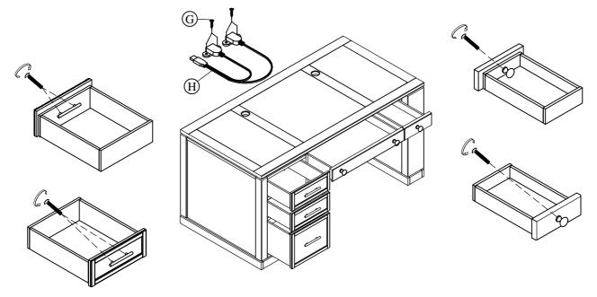
Open the pullout drawer, take off the handle & knobs installed on the back of drawer front and reattach the handle on the front side as shown.
