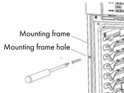
2. There are two holes, one on each side of the front frame that surrounds the oven cavity. Drill 1/8" (3.18 mm) pilot holes through the holes, and into the front wall of the cabinet. There are four mounting holes, two on each side.
