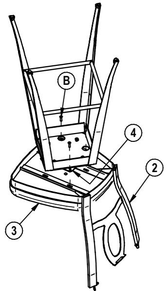
6) Insert the wooden or upholstered backrest on the frame. Screw it on with **E** screws beginning with the center ones.
