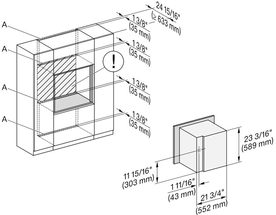
**A** Cutout (min. 28 sq in/18,000 mm<sup>2</sup>) for power cord and ventilation
