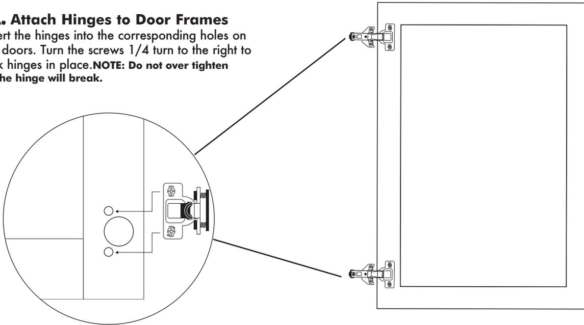
**Note: The hinge can be separated by pulling the black tab and pulling apart the hinge from the hinge base. Separated hinges snap back together.**
