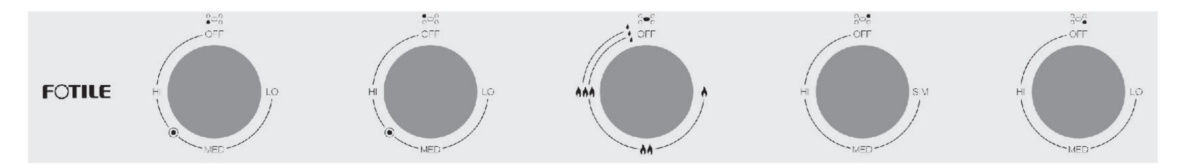
Turn the control knobs to adjust the flame level. Turn the knob counterclockwise, 90° for high flame, 180° for middle flame, and 270° for low flame. Check below table for different BTU between high/middle/low flames.
