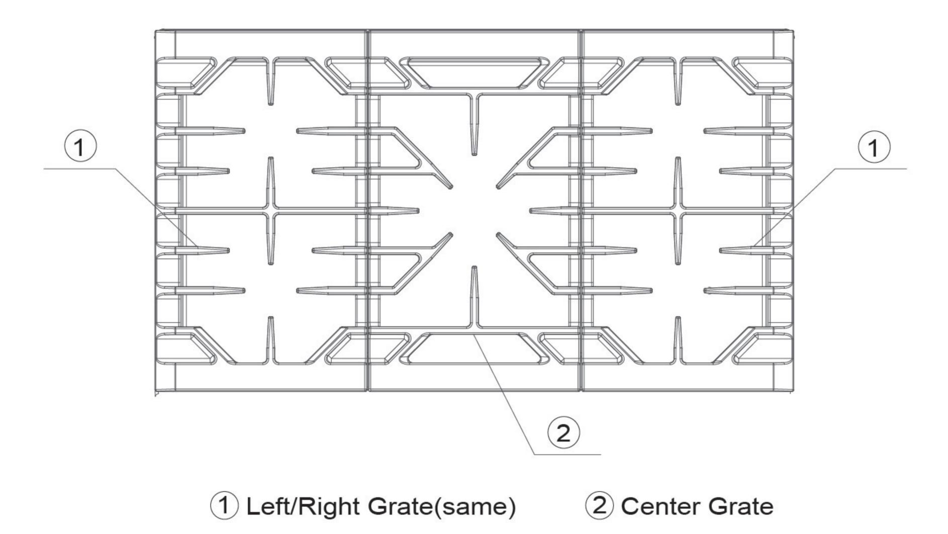
The three cooktop grates are designed to fit in specific positions on the cooktop. For maximum stability, these grates should only be used in their proper positions.
