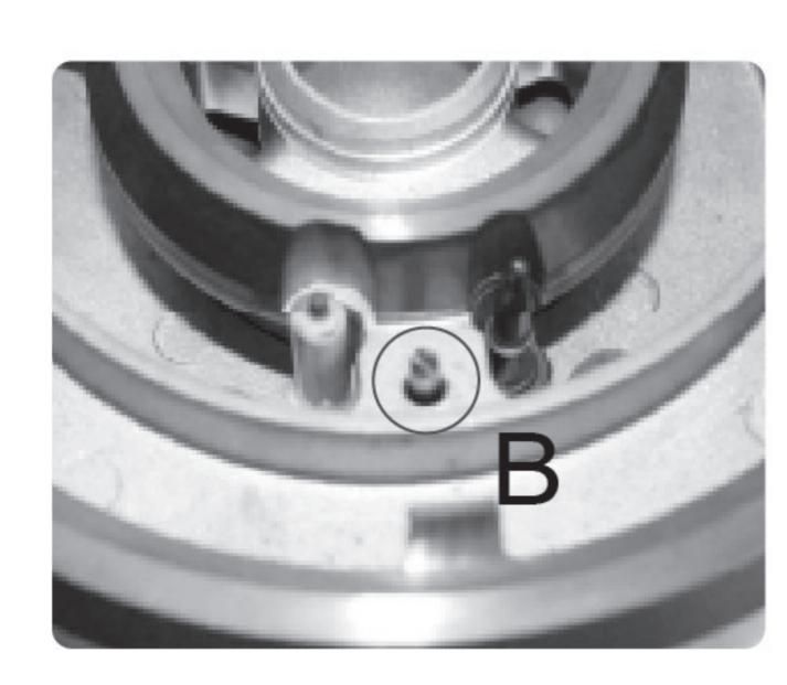
3. Place the lined part of outer burner cap to fit in the lined part of the burner head. Shake the outer burner cap gently to check if it is firmly seated (you will be able to rotate the outer burner cap, but it should be firmly seated in the burner head.)
