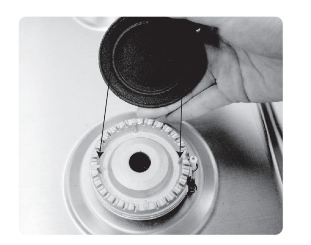
5. Check if the burner head/burner cap is firmly seated. If the burner head/cap is not level or is unstable, you must take it off, and reinsert it again.
