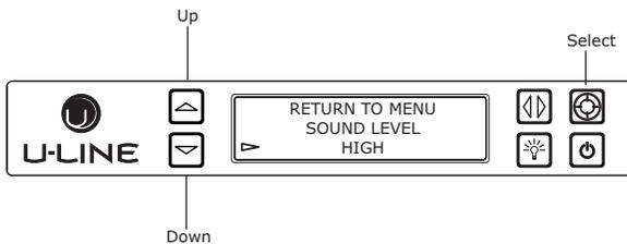
Audible alarms and alert tones support four different Sound Level settings, High, Medium, Low, and Off.
