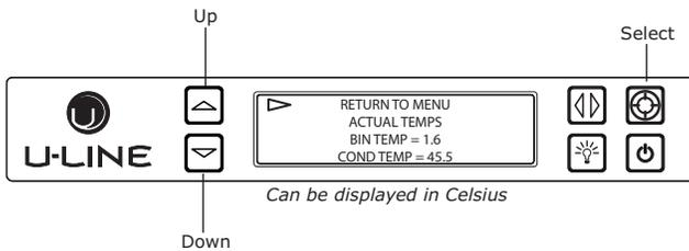
The Actual Temps option displays the actual temperature of the ice bin and condenser, as well as ambient temperature.
