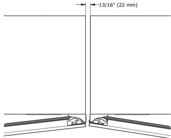
Stainless steel models which include the standard stainless handle will require 4-9/16" (116 mm) to allow both doors to open to 90° at the same time.
