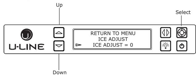
The Ice Adjust option adjusts ice thickness by adding or subtracting up to 5 minutes of ice production.
