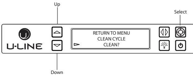
A clean cycle can be initiated through this menu. Once the cleaning cycle starts, the cycle cannot be stopped until complete.
