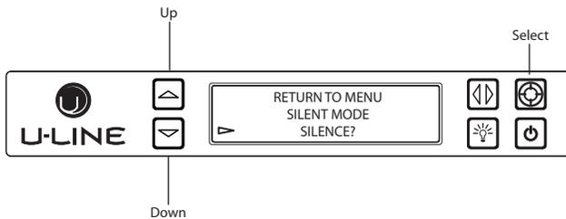
Users can halt ice production for 3 hours with an option called “Silent Mode” in the Customer Menu. Silent Mode will begin once the current ice making cycle is complete. After 3 hours in Silent Mode, normal ice production will continue.
