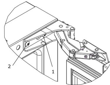
**Note: One hinge includes a metal spacer. Spacer must be used with that hinge when reversing the door.**
