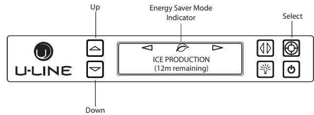
Energy Saver mode reduces overall energy consumption by reducing the amount of ice stored in the bin, along with decreasing the lighting.
