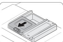
1. Gently press the dispenser flap to unlock, and then slide it open. Note that the dispenser flap opens at the end of each cycle.
