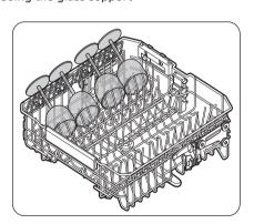
The glass support is especially suited for wine glasses. Hang wine glasses onto the pegs of the glass support. Fold the glass support back when it is not being used.
