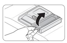
1. Pull up the cap of the rinse compartment to open.
