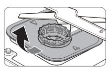
**3.** Remove the filter cover, and then the cylindrical micro filter underneath.
