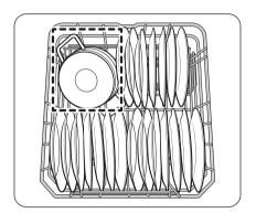
For more effective cleaning, load large items into the Storm Wash+ area on the left side of the lower rack (Dotted zone). When you select Storm Wash+, the
