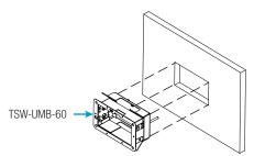
2. Loosen the two screws on the included TSW-UMB-60 universal mounting bracket, and then install the TSW-UMB-60, bottom first, into the opening.
