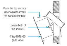
3. Reach into the TSW-UMB-60 and push the rear half back to ensure it is fully behind the mounting surface. Ensure the front of the TSW-UMB-60 is level, and then tighten the two screws to complete the installation.
