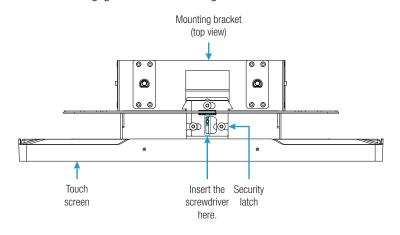
NOTE: There is a small amount of "play" in the bracket mounting, which allows room to insert the screwdriver.
