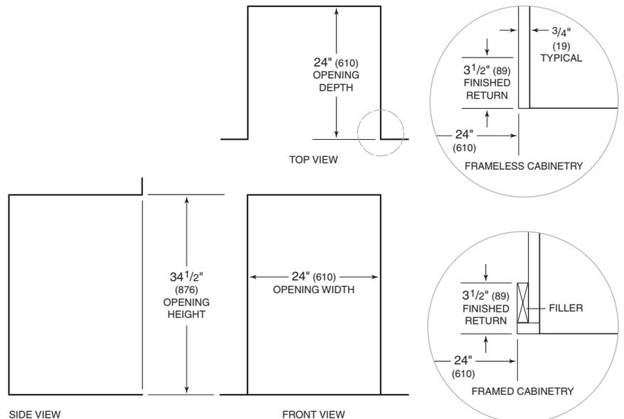
NOTE: 3<sup>1</sup>/<sub>2</sub>" (89) finished returns will be visible and should be finished to match cabinetry.
