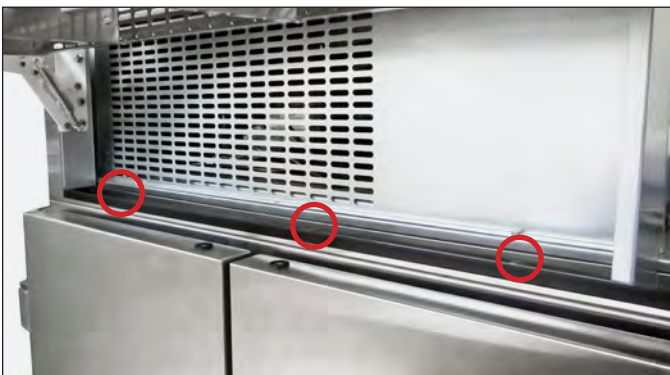
FIG. 9. Rainshield screw locations.
