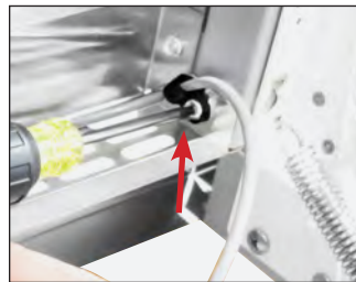
FIG. 6. Remove the p-clip holding the wire to the rainshield.
