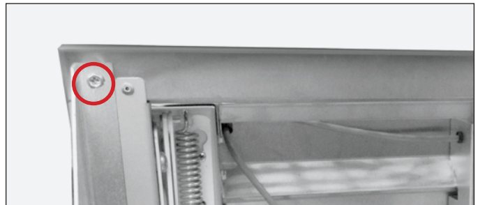
FIG. 8. Bracket screw location. Other bracket not shown.
