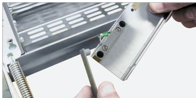
FIG. 4. Remove the plastic cover.
