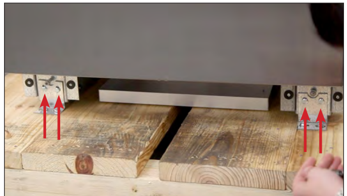
FIG. 7. Shipping bracket bolt locations.
