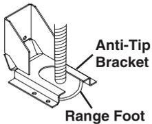
To verify the anti-tip bracket is installed and engaged:
