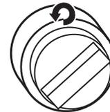
If the burner does not light, check cap alignment. If the burner still does not light, do not service the sealed burner yourself. Contact a trained repair specialist.
