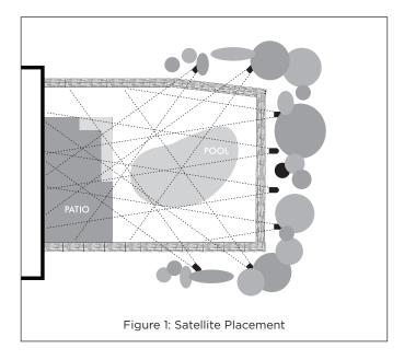
Use care to select satellite locations that are equally distant from the main listening area. When possible, use high and low locations to centralize the acoustic stage (see Figure 2).
