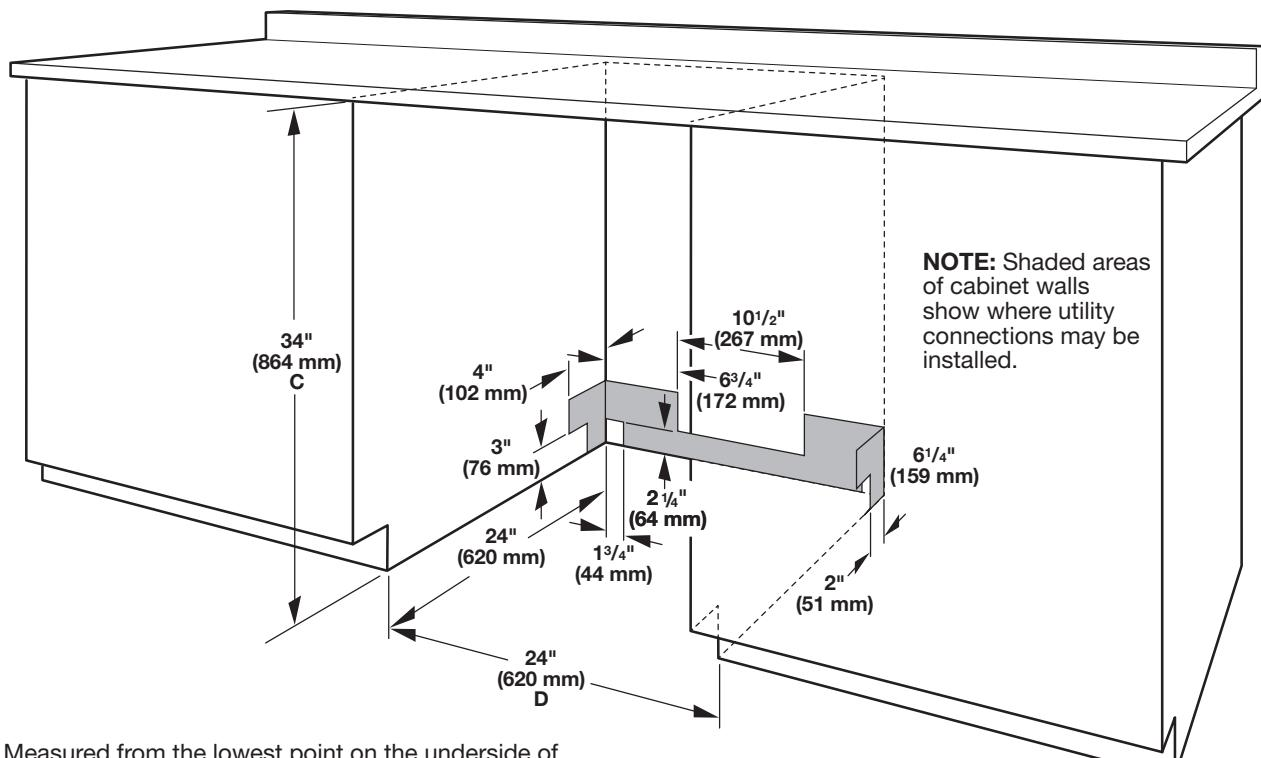
C. Measured from the lowest point on the underside of the countertop. May be reduced to 33 1/2" (851 mm) by removing the wheels and perforated area of insulation (blanket) on dishwasher.
