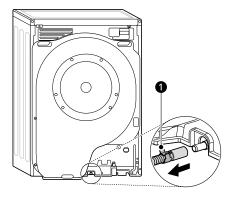
Connect the drain hose of the dryer and secure the hose clamp.
